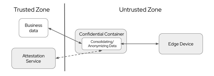
Securing privacy data from external access in an edge device.
