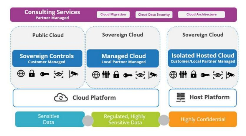
**Sovereign Controls**: Built-in platform controls offered by the public cloud provider, which the customer manages. These controls include data residency, encryption/key management, and access management.
